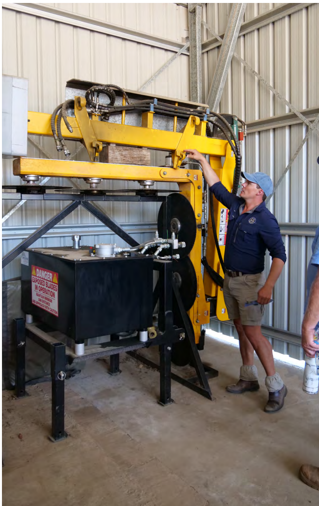
Jan's specialised rotating hedger for pruning individual trees.
