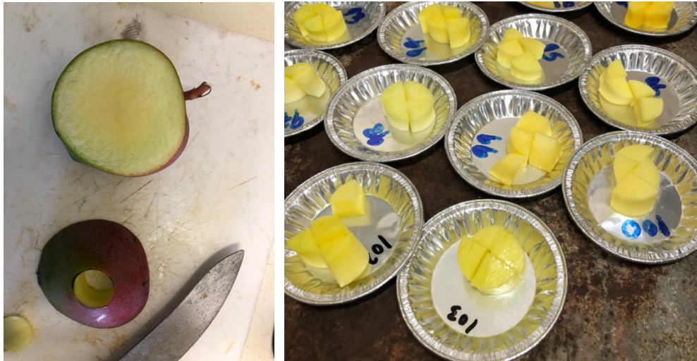
Figure 1. For best results, samples should have a weight of 7 to 10 grams. Samples taken with a corer are usually cut in four.
